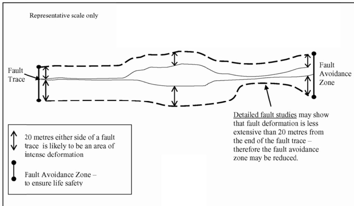
**Figure 13** A fault avoidance zone on a district planning map (from Kerr et al. 2003). Note that following specific targeted geological or surveying work, the Fault Avoidance Zone width can be decreased to allow buildings closer to the fault trace.
