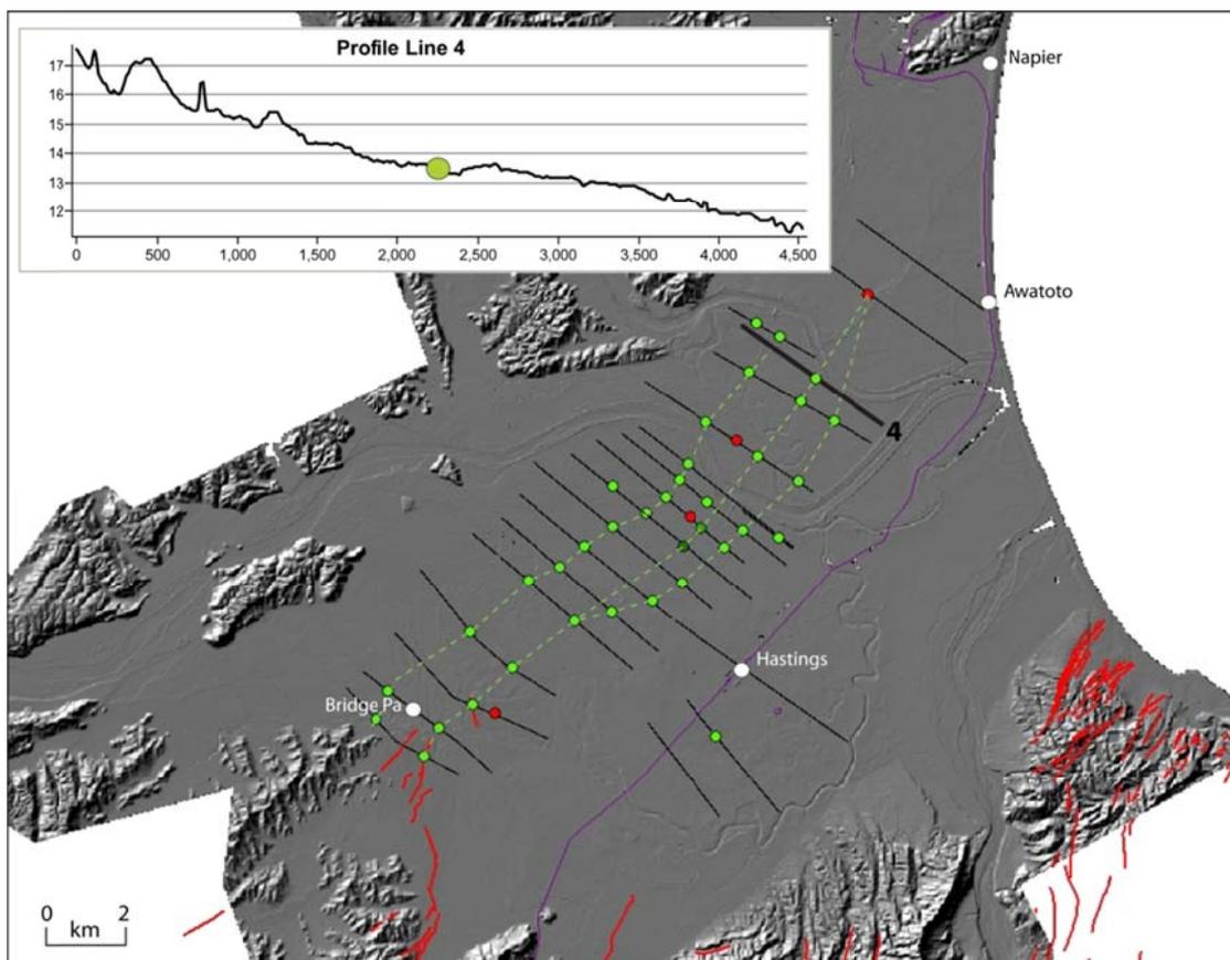
**Figure 12** LiDAR DEM of the Heretaunga Plains and surrounding area. The locations of active fault traces are shown in red. Black lines represent profiles made on the hillshade model perpendicular to the NE-trending structural grain. Green and red dots represent inflection points in the profiles where there is a significant change in gradient or slope direction. The green dashed lines attempt to link these together. Inset: Profile 4 at the Northeastern end of the Heretaunga Plains.
