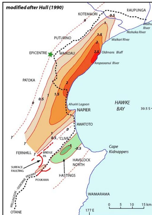
**Figure 11** Map of vertical deformation and surface faulting (thick red lines) related to the 1931 Hawke's Bay earthquake as interpreted from the re-levelling of the local rail network (after Hull 1990). Uplift is shown in orange colours and subsidence in green.
