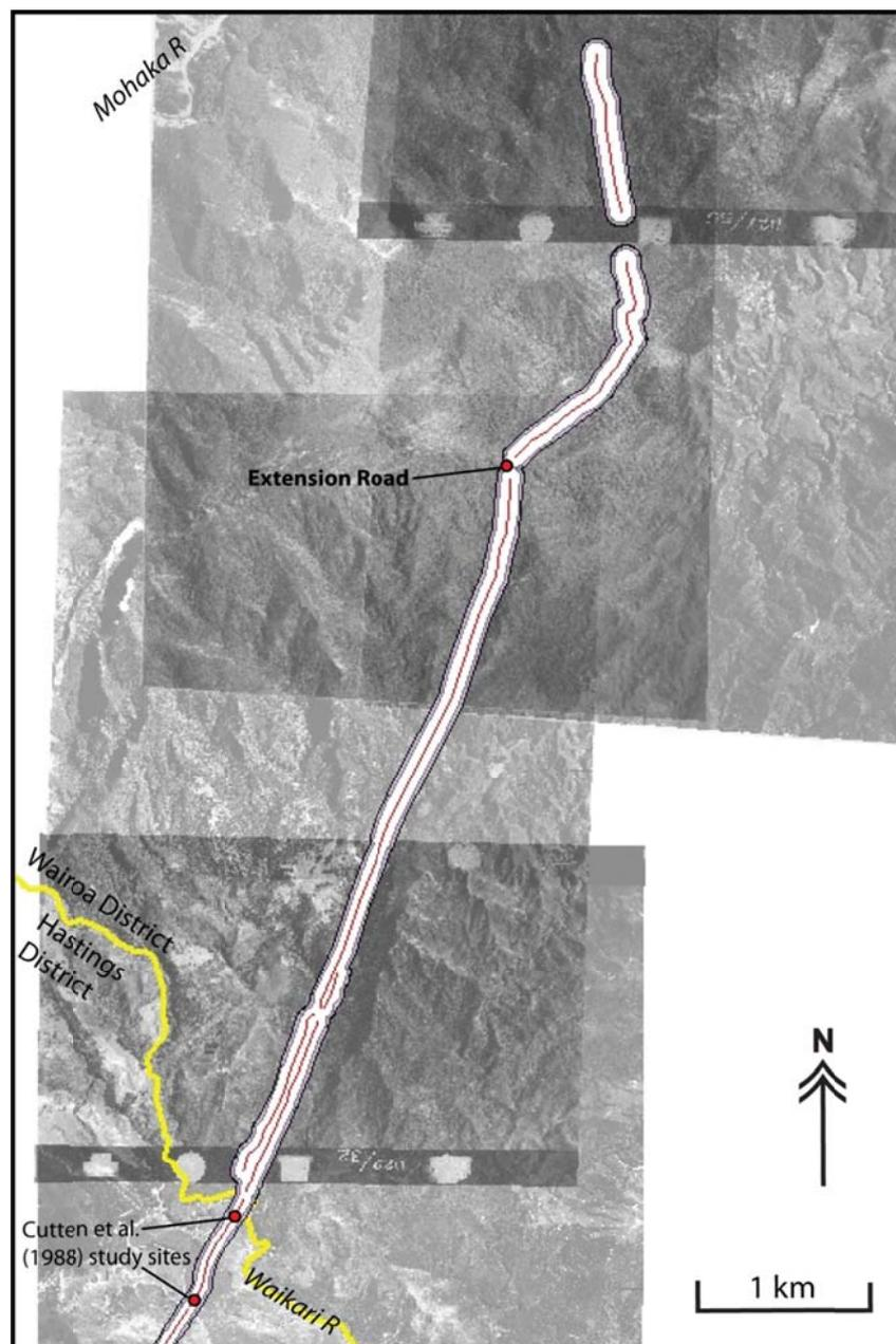
**Figure 10** Fault mapping using georeferenced aerial photographs in a GIS. In this example, the northern end of the Rangiora Fault in Wairoa and Hastings Districts is shown with its Fault Avoidance Zone. The total width of the FAZ includes a margin of safety buffer of  $\pm 20$  m (about the white buffer).
