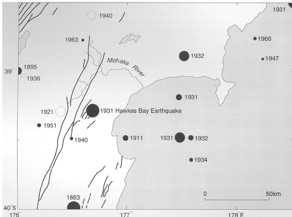
**Figure 8** Map of the Hawke's Bay region showing large historic earthquakes. The epicentre of the 1932 M 6.9 Wairoa earthquake is shown near the top centre of the image (figure from Cutten 1994).
