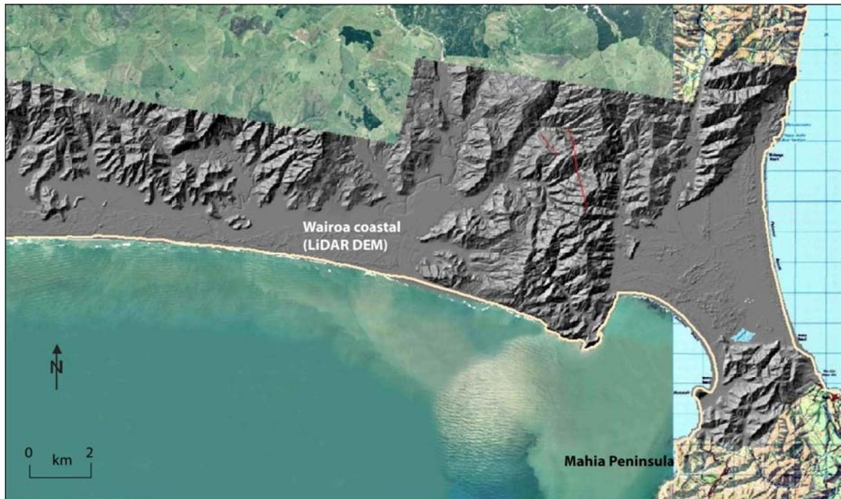
**Figure 4** LiDAR shaded hillslope map of a portion of the Wairoa coastal area (grey DEM). Red lines represent active faults within the GNS Science Active Faults database prior to this study. The 1-m DEM has allowed us to revise this mapping, so that no active fault traces are now identified.
