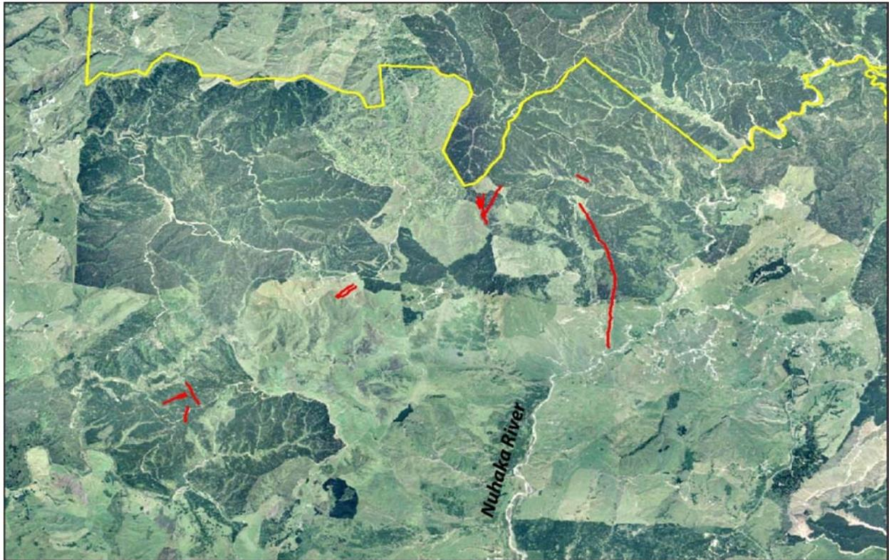
**Figure 6** Orthophotograph of part of Wairoa District in the area of the upper Nuhaka River. The yellow line represents the northern boundary of Wairoa District. Red lines represent updated fault linework (possible active fault traces) for this area. The GIS data with Fault Avoidance Zones from the accompanying CD should be used to characterise this line data.
