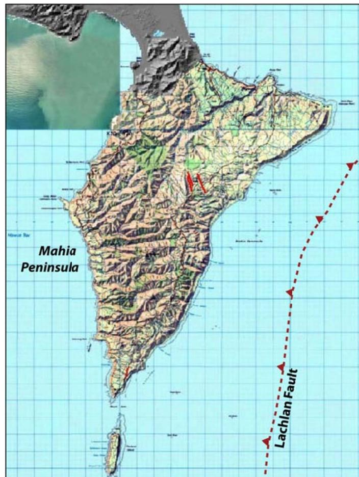
**Figure 9** Map of Mahia Peninsula with the previous locations of active fault traces in red. No LiDAR or orthophotograph coverage exists over the majority of the peninsula. The approximate location of the Lachlan Fault, an important offshore reverse fault is shown to the east of the peninsula.
