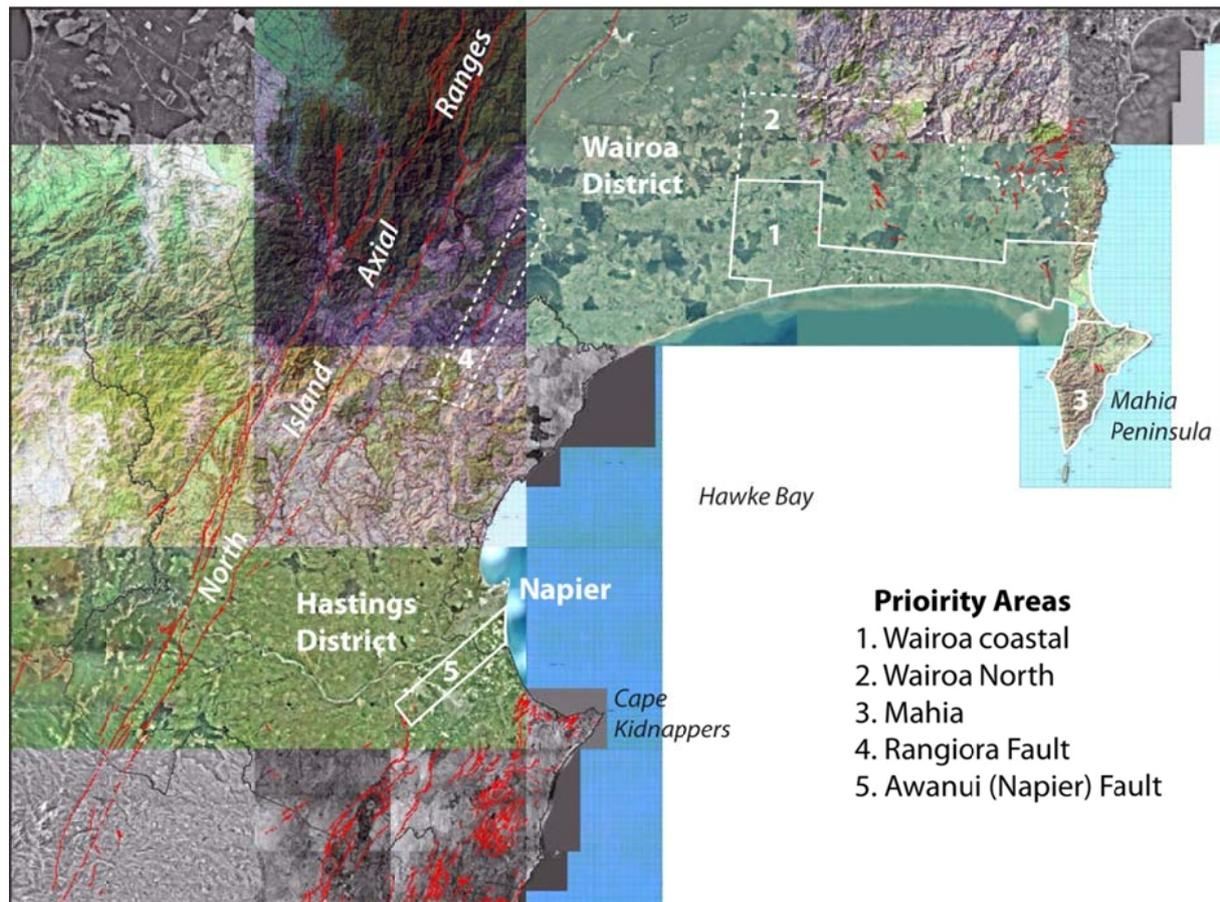
**Figure 3** Orthophotograph coverage of northern Hawke's Bay. The priority mapping areas are shown by white polygons. Active faults from the GNS Science Active Faults database are shown in red. Area 1 is defined by a strip of LiDAR data flown in the coastal part of Wairoa District.
